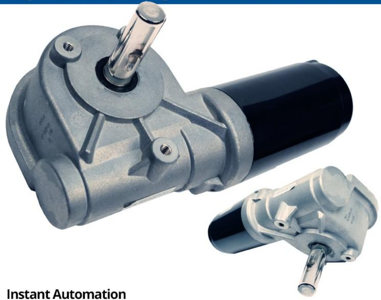
Lightweight and self-contained, Superwinch® Power Drives are the ultra-dependable, high-quality solution for many applications requiring a prime mover for task automation. Designed with longevity in mind, Superwinch uses only oversized bearings, substantial wormshaft and a high-end tin-bronze alloy worm wheel for the utmost in durability.
