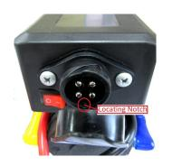
The BC3500 solenoid control box has a 4 pin sock with locating notch. This is used for all plug in control options.. The socket is suitable to accept the corded hand held control or the wireless receiver.
