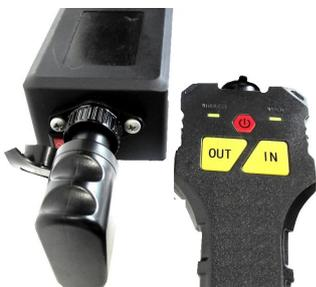
Wireless receiver plugs into the control box
