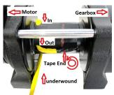
The BC3500 is suited to both steel or synthetic rope. In either installation the rope is fed under the drum from the front of the winch and then into the drum from behind the winch. This is correct with the motor on your left and gearbox on your right when facing the winch. Incorrect rope attachment will not allow the brake to function correctly and support loads..
