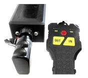
Wireless receiver plugs into the control box
