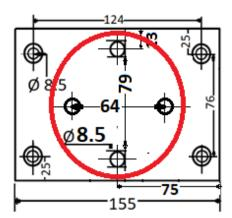
The bolts must be secured with spring washer behind the nut or lock nut should be used. Two flat washers should be used on the bolts on both sides of the mounting plate one under the bolt head and one under the lock washer or lock nut. Ensure all nuts are firmly secured at 30 Nm of torque for M8.
