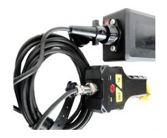
The Wireless transmitter can become a 4 metre corded control when required or if preferred. There is a Wired Lead In adaptor at the top of the transmitter. Remove the cap to expose a locating point which matches that of the cord. Once connected it has a threaded locking sleave for retention. The opposite end will plug into the control box socket, also use the locking sleave to secured into position.
