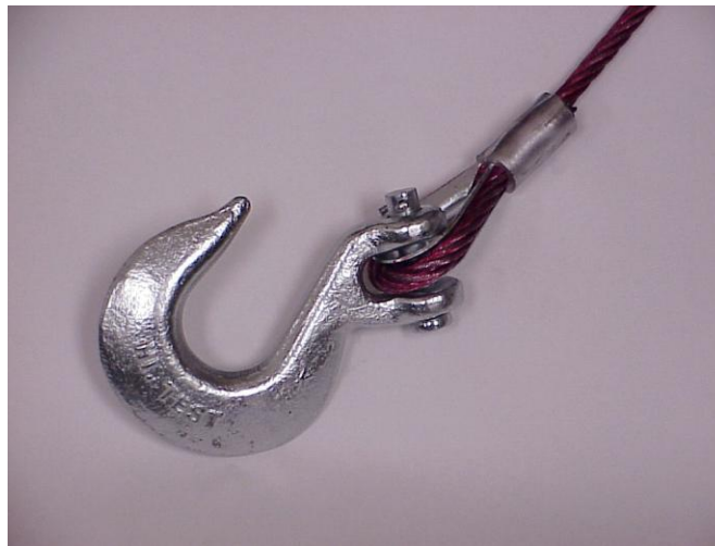
A properly installed hook.
