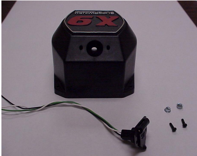
Solenoid Cover Socket Removal. ( old style socket PZQ93 00010 )
