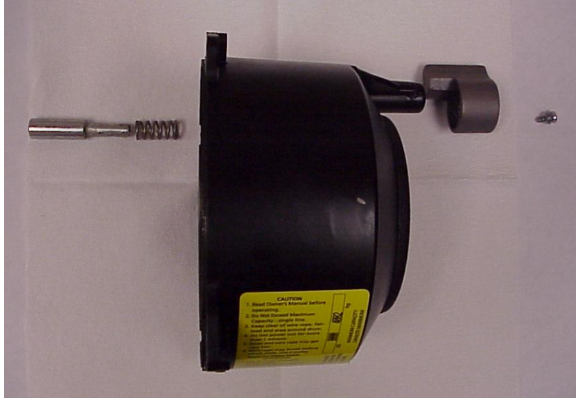
Freewheel knob and lock pin removal.
