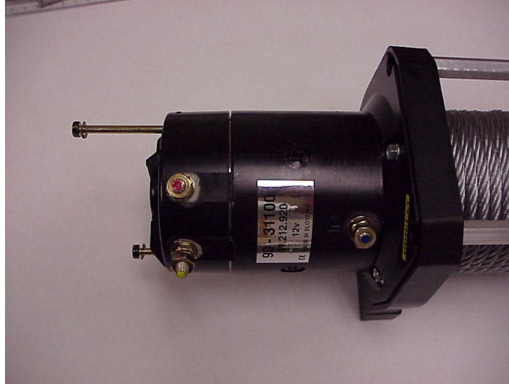
Motor mounting bolt removal.
