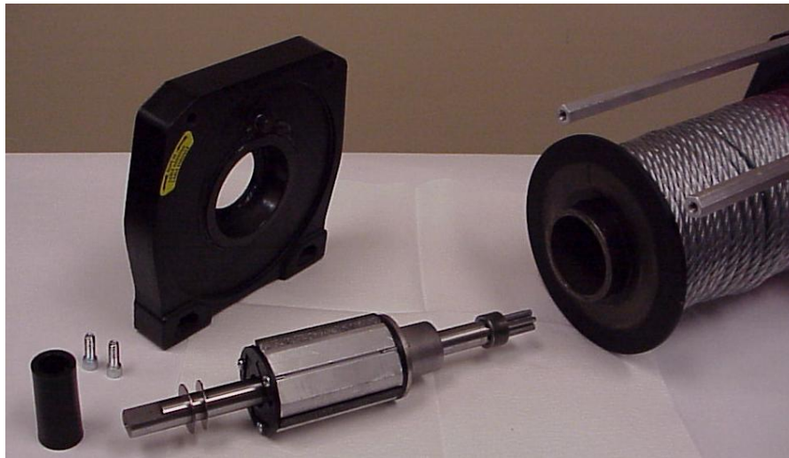
Brake and drive shaft removal shown from MOTOR end of the winch.
